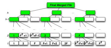
Fig. 3. Analysis of the tree of files created in multi-pass merge.
