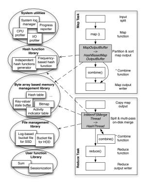
Fig. 10. Architecture of our new one-pass analytics platform.
