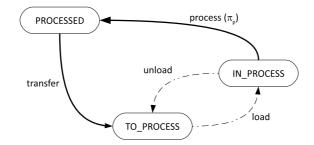
Figure 4: The Finite State Automaton modeling a product.
