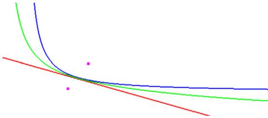
Fig. 2. Three Itakura-Saito bisectors: first-type (red), second-type (blue) and third-type (green). The first-type Bregman bisector is always a linear separator. (For interpretation of the references to color in this figure legend, the reader is referred to the web version of this article.)
