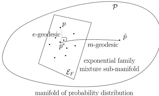
**Fig. 1.** Simplifying a statistical mixture of exponential families or KDE  $\tilde{p}$  to a single component model amounts to perform a Kullback-Leibler projection of the mixture onto the exponential family manifold [45]. Optimality is proved using the Pythagorean theorem of dually flat geometries.
