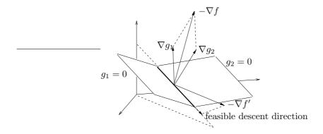
Figure 2: If  $\nabla f$  is linearly dependent on the constraint gradients, there is no feasible descent direction.  $\nabla f'$ , which does not have this property, identifies a feasible descent direction when projected on the feasible space.
