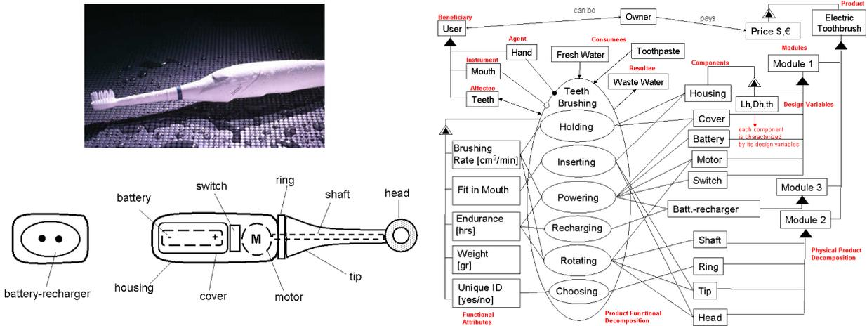
Figure 2: The battery-powered toothbrush product (left) and its object-process diagram — functions=ovals, objects=rectangles (right).
