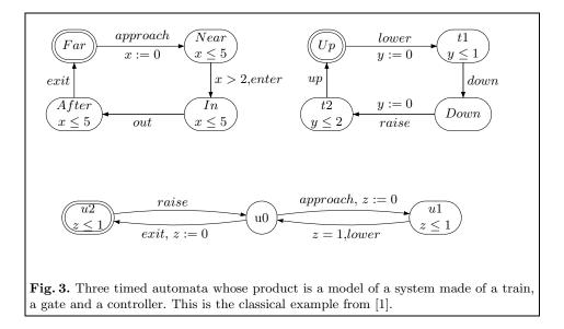
*Product construction.* Timed automata can be composed by *synchronisation* [1, 4] (see figure 3 for a classical example). Intuitively, building the product of two timed automata consists in considering a timed automaton whose state space is the product of the state spaces of the automata, where transitions labelled by a same letter in the two automata occur synchronously, and others may occur asynchronously.
