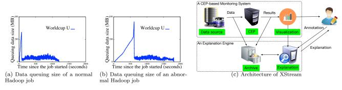
Figure 1: Hadoop cluster monitoring: examples and system architecture.
