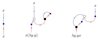
Here we can see that the leftmost diagram corresponds to the identity term, the middle diagram to a function-open term, and the rightmost diagram to a value-open term. Reading across the rows of the bottom half of Figure 5, we can quickly check that among the nine NPTs of size = 3, the first four are function-open and the next five are value-open.
