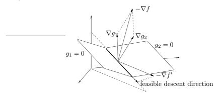
Figure 12: If  $\nabla f$  is linearly dependent on the constraint gradients, there is no feasible descent direction.  $\nabla f'$ , which does not have this property, identifies a feasible descent direction when projected on the feasible space (the thick line).
