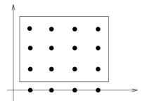
Figure 17: Projecting a grid distribution in  $\mathbb{R}^2$  on the coordinate axes reduces the number of projected points. In this picture, N = 12 but the projected points are just 4.
