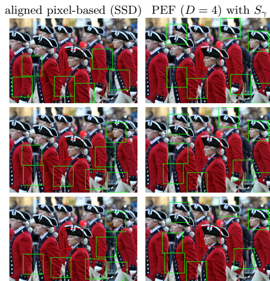
Fig. 1. Comparison of PEFPM with the baseline SSD patch matching (patch size 150 \times 150 and image size 960 \times 640 ): Observe that due to its flexibility the statistical modeling got more face hits (4 faces) than the pixel-aligned SSD method (one face). The upper row is on pixel intensities, the middle row on sum of RGB channel dissimilarities, and the last row on the maximum of RGB channel dissimilarity.
