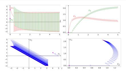
The controller leads the output  $(x_3, x_4)$  to the desired position (1, 2)
