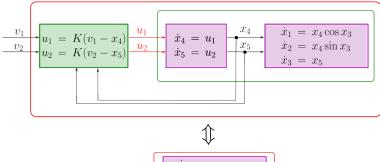
$$\begin{array}{c|c} v_1 \\ \hline v_2 \\ \hline v_2 \\ \hline \end{array} \begin{array}{c} \dot{x}_1 = v_1 \cos x_3 \\ \dot{x}_2 = v_1 \sin x_3 \\ \dot{x}_3 = v_2 \end{array}$$
