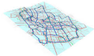
Figure 2.17: Optimization of water networks: deciding diameters for all pipes and water flow given water at each node over a time horizon [Bragalli et al., 2012]. Although this is actually a nonconvex cMINLP methods are used heuristically to solve it.
