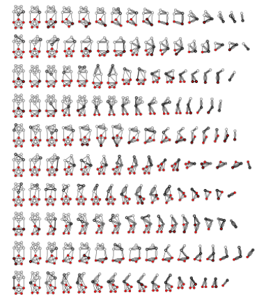
Figure 5.2: Karger’s randomized algorithm for MIN CUT contracts edges at random until only one edge remains — which corresponds to a cut in the original graph. This extremely simple algorithm returns a minimum cut with probability 2/(n(n-1)) (where n = |V| ), which is much better than the one obtained by sampling a cut at random (from Wikipedia). Unlike MAX CUT, however, a polytime algorithm for MIN CUT is known (Which one?) — this goes to show that randomized algorithms can sometimes also be useful for problems which we can solve “efficiently” (it all depends how one defines this term!). Write a Python code to evaluate whether the Karger’s algorithm is better or worse than a deterministic MIN CUT algorithm, on a significant test set.
