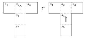
Also, the following two states are distinguishable for the robot, because it can distinguish between having an open space in front of it or behind it:
