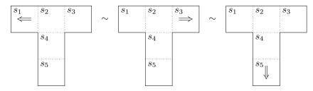
The following two states, however, are distinguishable, because in the first one, the robot perceives that there is only a wall in front, while in the second one it perceives that there are walls on either side:
