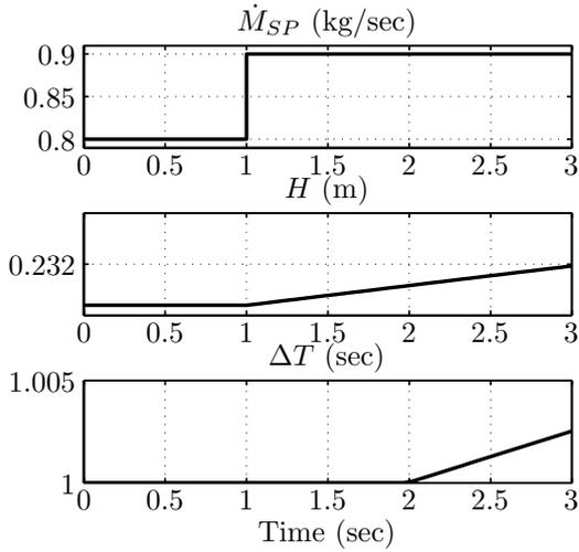
Fig. 5. Step response for  $\dot{M}_{SP}(t)$ ,  $\Omega_R(t) = \text{const}$ , of the operation point. By keeping the force constant, which is a gage of constant quality, the demand can be to change the thickness  $D_B(t)$  of the strip or to change the amount of produced steel strip per hour. This decoupling problem is formulated in (Simon, 2000) as follows. Is it possible to change the operating point by keeping the force  $F(t)$  constant such that
