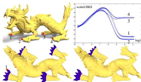
**Figure 1:** top left: dragon model; top right: scaled HKS at points 1, 2, 3 and 4. all four signatures are close at small  $t$ 's while big  $t$ 's separate the points on the front claws from those on back; bottom left: the points (blue), whose signature is close to the signature of point 1 based on the smaller half of the  $t$ 's; bottom right: based on the entire range of  $t$ 's.
