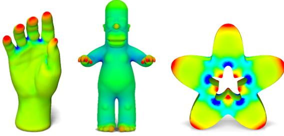
**Figure 3:** Heat kernel function  $k_t(x, x)$  for a small fixed  $t$  on the hand, Homer, and trim-star models. The function values increase as the color goes from blue to green and to red, with the mapping consistent across the shapes. Note that high and low values of  $k_t(x, x)$  correspond to areas with positive and negative Gaussian curvatures respectively.
