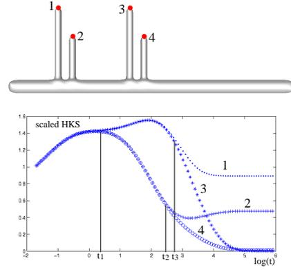
**Figure 5:** Top: a synthetic model; bottom: the scaled HKS corresponding to the four marked points.
