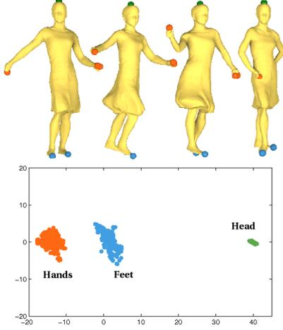
**Figure 10:** Top: Feature points on 4 models in the dataset by Vlastic et al. [VBMPO8]. Bottom: the MDS embedding of the feature points from all 175 models based on their Heat Kernel Signatures at medium scales.
