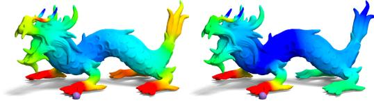
**Figure 6:** Color plot of the difference between the HKS defined by the range of scales  $[t_1, t_2]$  of the point marked by the purple sphere and the signatures of other points on the shape. The difference increases as the color changes from red to green to blue. left: both  $t_1$  and  $t_2$  are small; right:  $t_1$  is small, while  $t_2$  is large.
