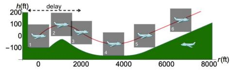
Fig. 4. Trajectory of the ownship (red) and safe region for the intruder (green), delayed response describes a *delay parabola*, in red on Fig. 4, and its position  $(r_t, h_t)$  along the nominal trajectory for  $0 \le t < d$  is given by  $(r_t, h_t) = \left(r_v t, -\frac{a_d}{2} t^2 + \dot{h}_0 t\right)$ .
