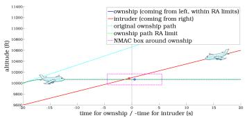
Fig. 7. Original ownship path (cyan) and intruder path (red) vs. ownship responding to a donot-climb (DNC) advisory (green dotted line) issued by the ACAS X tables in starting state:  $r = 4,000 \text{ ft}, r_v = 200 \text{ ft/s}, \theta_v = 180^\circ, h = 600 \text{ ft}, \dot{h}_0 = 1,980 \text{ ft/min}, \dot{h}_1 = -1,500 \text{ ft/min}.$
