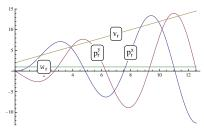
(c) Position  $(p_r^x, p_r^y)$ , translational velocity  $v_r$  and rotational velocity  $\omega_r$  for translational acceleration on a spiral.
