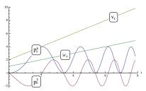
(a) Position  $(p_r^x, p_r^y)$ , translational velocity  $v_r$  and rotational velocity  $\omega_r$  for positive acceleration on a circle.
