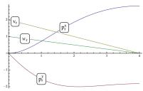
(b) Position  $(p_r^x, p_r^y)$ , translational velocity  $v_r$  and rotational velocity  $\omega_r$  for braking to a complete stop on a circle.
