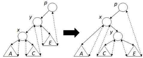
Fig. 1. Logical ordering tree. Following a right rotation of  $y$ , a traversal about to navigate from  $y$  towards  $A$  (before) would normally reach  $C$  instead (after). However, it can follow *pred* pointers (dashed) to reach  $A$  from  $C$ .
