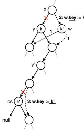
Fig. 7. Removing a node  $y$  with two children by creating a copy  $w$  of the node  $cs$  containing the smallest key  $k'$  bigger than the key  $k$  of  $y$  (the successor). Dashed edges represent changes of pointers made during this removal. They are labeled with integers that show their order and updates of the ghost field key.
