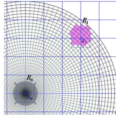
Figure 6. Remapping the points in polar coordinates to points in the grid
