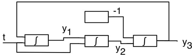
**Figure 2.** Generating cos and sin by a GPAC. In form of a system of equations, we have  $y_1' = y_3$ ,  $y_2' = y_1$ ,  $y_3' = -y_1$ . It follows that  $y_1 = \cos$ ,  $y_2 = \sin$ ,  $y_3 = -\sin$ , if  $y_1(0) = 1$ ,  $y_2(0) = y_3(0) = 0$ .
