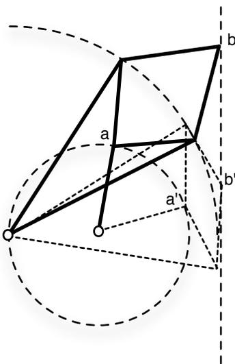
**Figure 4.** Peaucellier's mechanism. The circular motion of  $a$  is transformed into a linear motion of  $b$ .
