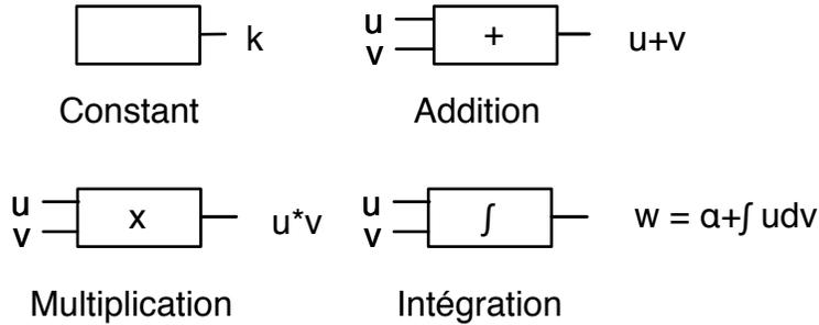
**Figure 1.** The basic units of a GPAC (the output  $w$  of an integration operator satisfies  $w'(t) = u(t)v'(t)$ ,  $w(t_0) = \alpha$  for some initial condition  $\alpha$ ).
