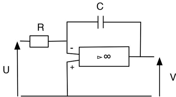
**Figure 3.** Realizing an integration with an ideal operational amplifier: one has  $V(t) = -1/RC \int_0^t U(t)dt$
