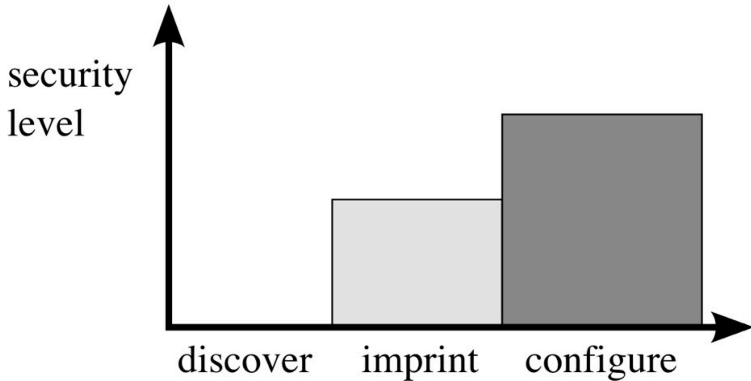
Fig. 2. Increasing security level along the bootstrapping process
