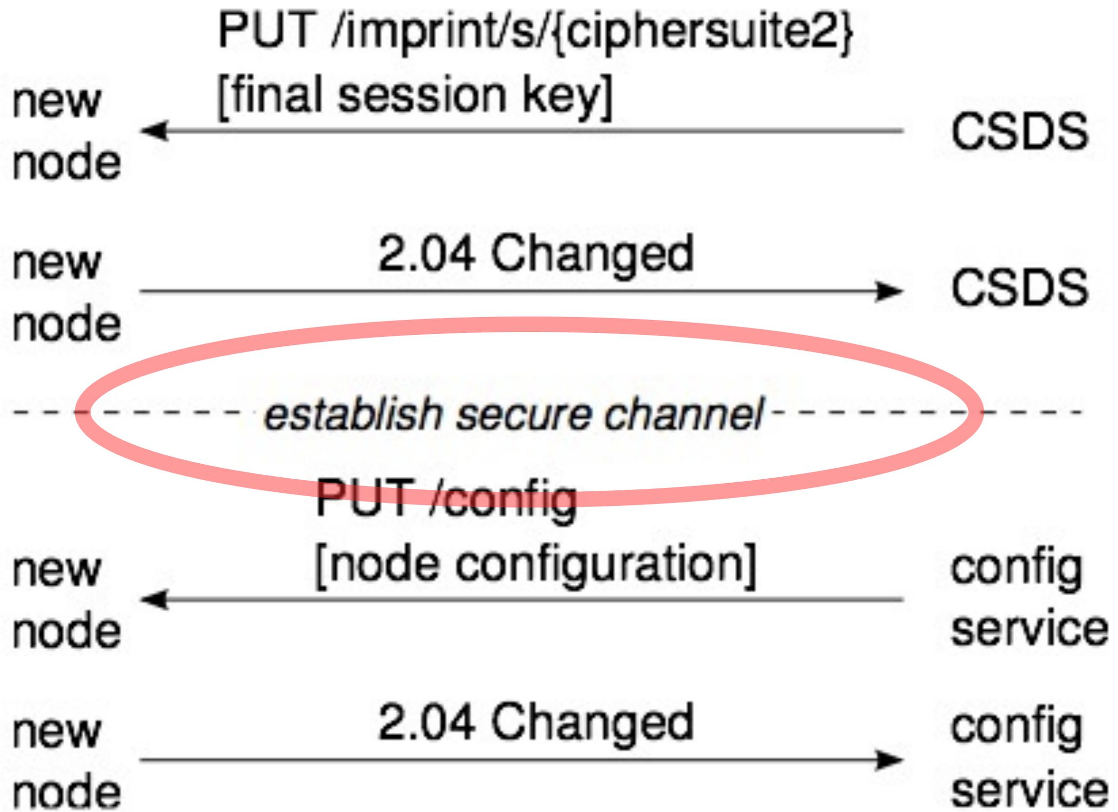
Fig. 5. Imprinting the final session key and configuring the new node
