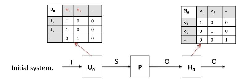
Given an input randomization  $U_R$  and an output randomization  $H_R$  such that  $U_R \circ P \circ H_0 = U_0 \circ P \circ H_R$  the following holds:
