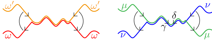
FIGURE 10. A schematic representation of kissing and non-kissing walks. The walks \omega and \omega' kiss (left) while the walks \mu and \nu share a common substring but do not kiss (right). Illustration from [PPP17].
