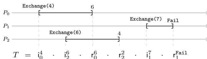
The trace  $T$  consists of *invocation* events  $i_i^x$  meaning that the object was called by process  $i$  with input  $x$ , and *response* events  $r_i^y$  meaning that process  $i$  returned with output value  $y$ .
