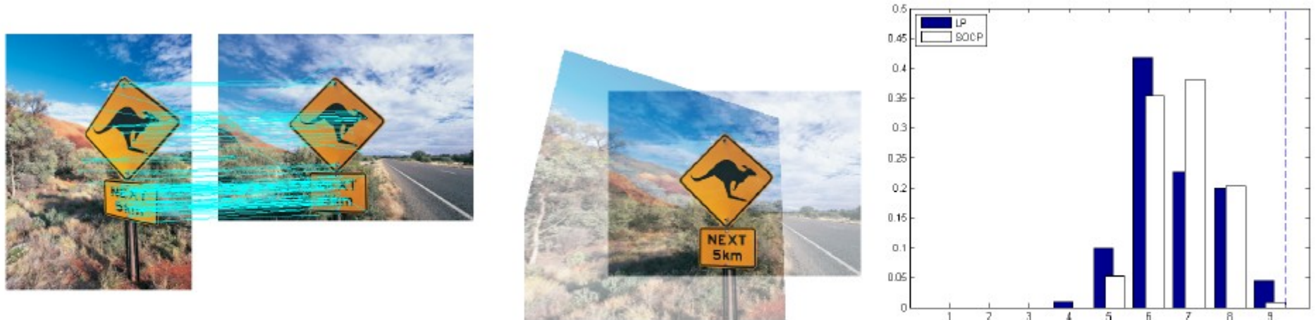
Figure 2. Left: A pair of images of a road warning sign with candidate matches found using SIFT descriptors. Middle: Resulting homography estimated using the dual SOCP approach. Right: Histogram of the number of measurements removed at each iteration using LP and SOCP formulations.
