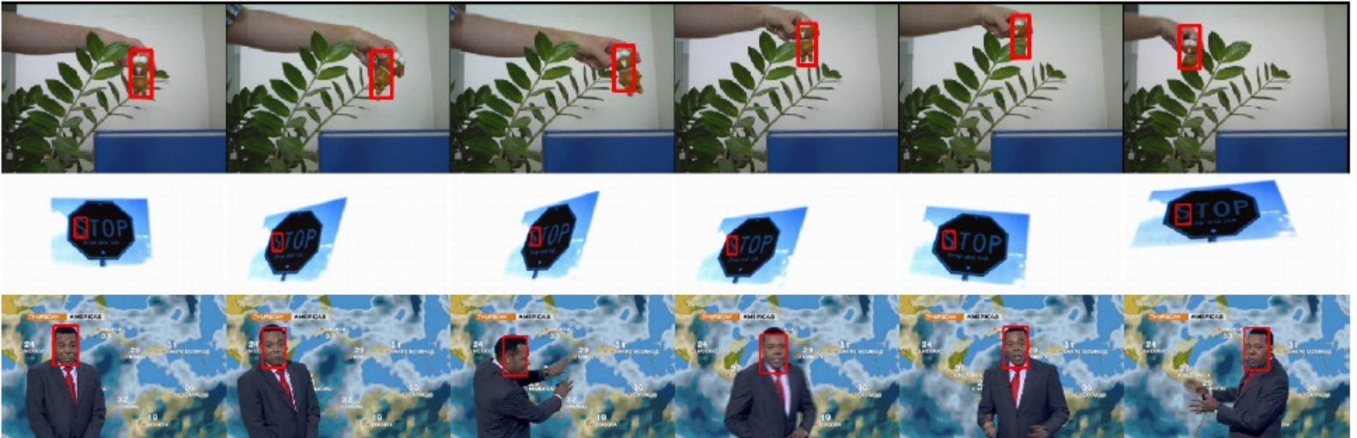
Figure 2. Object tracking using structure tensor as local descriptor. The tracker is manually initialized by drawing a bounding box over the object-of-interest in the first frame.
