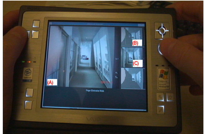
Fig. 5. Snapshot of our autoframing prototype application demonstrating the automatic finger elimination mode for the corridor test image: (a) source image, (b) segmented image with finger detected and region-of-interest box highlighted, and (c) suggested cropped picture.
