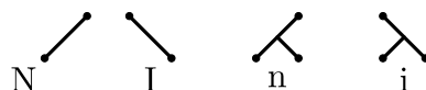
Figure 3: We label leaves of a binary tree by “N” and “I” as shown. Similarly we label the internal nodes by “n” and “i”. By convention we always label the root node “n”.
