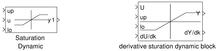
Figure 14: Saturation Dynamic block (left) and its derivative (right)
