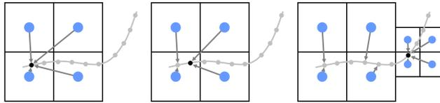
Figure 4: Adaptive grid sampling. The geometry points are processed sequentially (from left to right) and a deformation node is created if necessary in the 8 surrounding grid cells. The black dot indicates the current geometry point. The blue dots are nodes, the arrows point towards the anchor points of the nodes. Anchors are updated for each node to the nearest geometry point. Adaptive sampling creates nodes in smaller grid cells where necessary.
