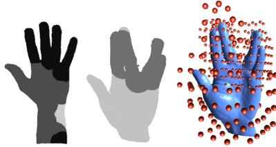
Figure 8: Weights computed by our adaptive sampling strategy for data sets hand-1 and hand-2, and the corresponding sampling. The color corresponds to the factor with respect to the base sample spacing. White means 1.0 (no increase in sampling), light gray 0.5 (two-fold oversampling) and dark gray 0.25 (four-fold oversampling).
