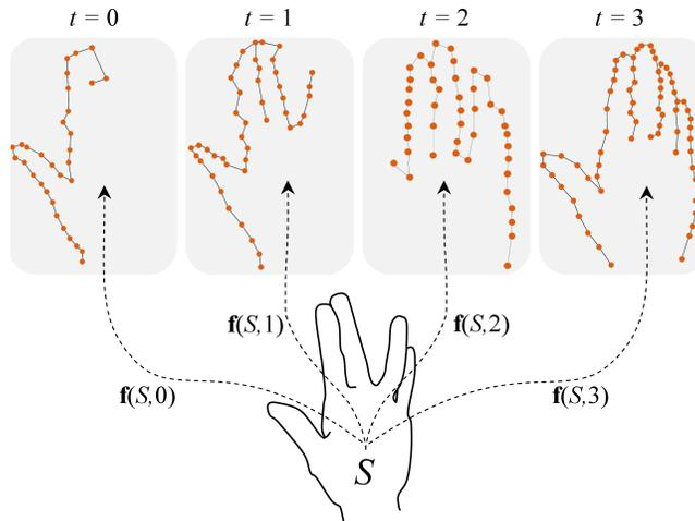
Figure 2: The goal in this paper is to construct one urshape  $S$  that represents the geometry of the object and a sparse, but adequate, deformation field  $\mathbf{f}$  that properly aligns the urshape to the input data. The urshape  $S$  and the deformation field  $\mathbf{f}$  are the output of our algorithm and completely define the shape and motion of the acquired object.
