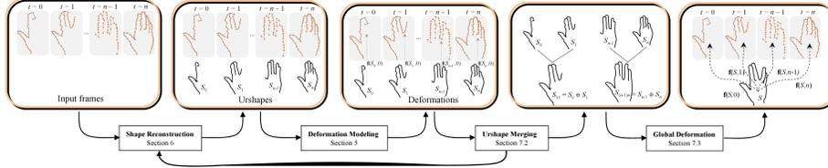
Figure 3: Animation reconstruction pipeline. From the initial input frames, our algorithm first computes urshapes. Next, smooth deformation fields are computed for each sequence. These deformation fields are used to merge adjacent sequences, resulting in updated urshapes that are fed back into the shape reconstruction pipeline until one global urshape and its deformation is found.
