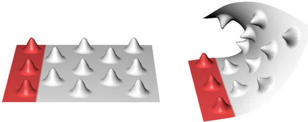
Figure 6: Example obtained using our meshless deformation algorithm. The red points are constrained, while the user deforms the geometry by pulling on one corner of the bumpy plane. As can be seen, the rigidity and volume preservation constraints are faithfully minimized using the non-linear solver and details are preserved during the deformation.
