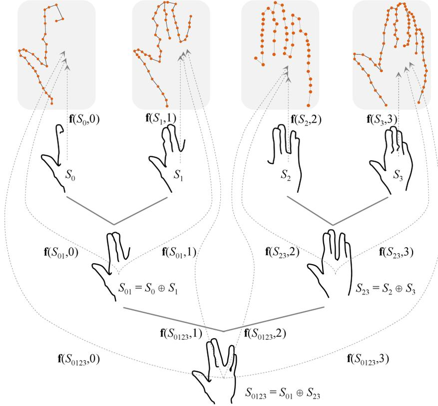
Figure 7: Hierarchical merging of sequences until a final urshape  $S_{0123}$  and a deformation field  $\mathbf{f}$  is obtained.
