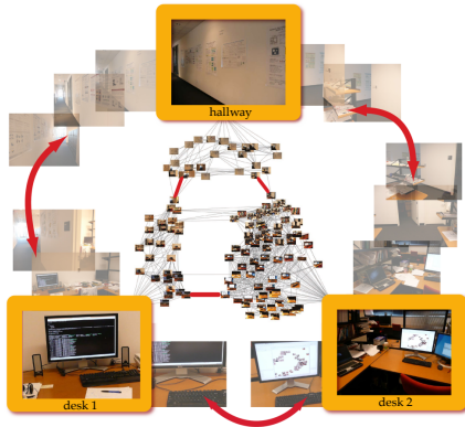
Figure 9. An image graph overlaid with detected landmarks (orange) and shortest paths between them. Edges marked in red correspond to the bottleneck edges between landmarks. Two paths between landmarks correspond to physical paths in the office while one path is caused by a shared object (keyboards on both desks).
