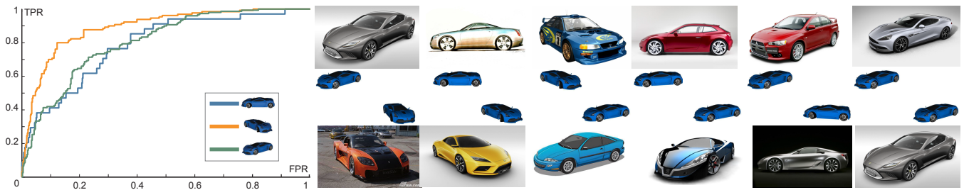
Figure 13: View-classifying Bing images using classifiers trained using 3D models. We assign a best view-estimate for each Bing image. Here, we show a set of example view estimations for ‘car’ images. The corresponding ROC curves are computed against ground truth data compiled by manually annotating each of the retrieved Bing images (only a sampling shown here).
