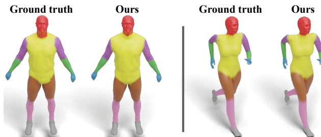
Figure 12. Qualitative evaluation of human shape segmentation on the dataset of [76]. Left: ground truth. Right: prediction by DiffusionNet + VADER.
