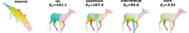
Figure 3. Previous methods focus on improving map accuracy and do not have explicit control over the map smoothness. Here we show an example of a non-isometric pair. We report the Dirichlet energy ( E_D ) of maps after refinement by different methods.
