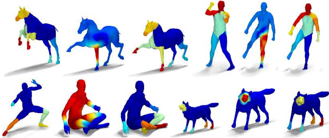
Figure 2.7: Segmentation transfer using the functional map representation. For each pair of shapes we show 3 figures: the user-provided source segmentation of the first shape, the image of one of the indicator functions of a segment using the functional map computed with our method, and the final segmentation transfer onto the target shape. Note that point correspondences were not computed at any point during this procedure.
