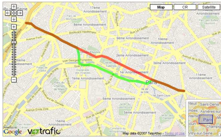
Figure 3: Picture of an application developed with the algorithm in Sect. 4.3: a path constrained to be within a guarantee region (red path, travel time: 5 minutes, 20 seconds) compared to the optimal solution (green path, travel time: 5 minutes, 12 seconds).
